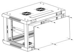
(5) Assemble the mounting bracket by 2pcs M4\*8 self-tapping screws.
