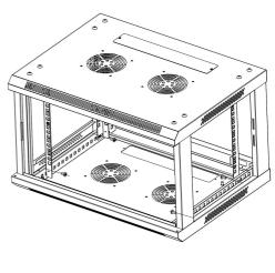
(3) Assemble the L type mounting brackets by 4pcs M6\*12 screws and 4pcs M6 cage nuts.
