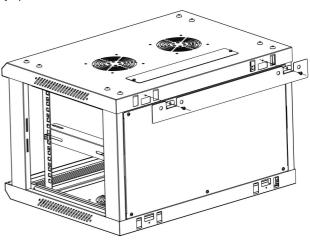
(6) Put the 1pc white plastic washer on the pin, then assemble the front door and 2pcs side panels to the unit.
