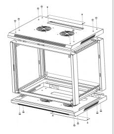
(2) Install the vertical rails by 8pcs M6\*12 screws and 8pcs M6 cage nuts
